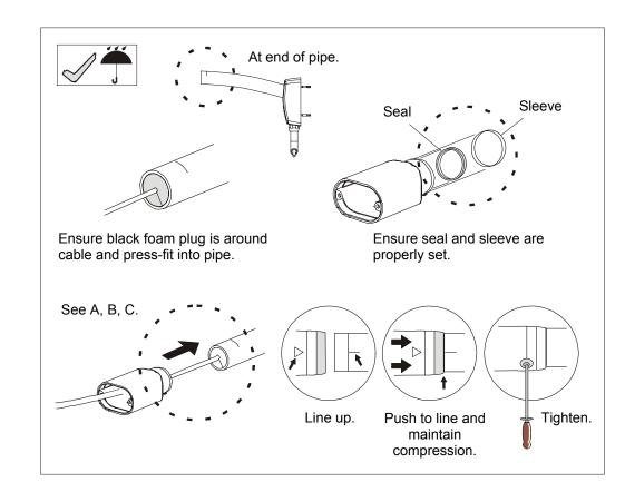
Thread cables through end cap assembly and attach housing to mounting structure.
